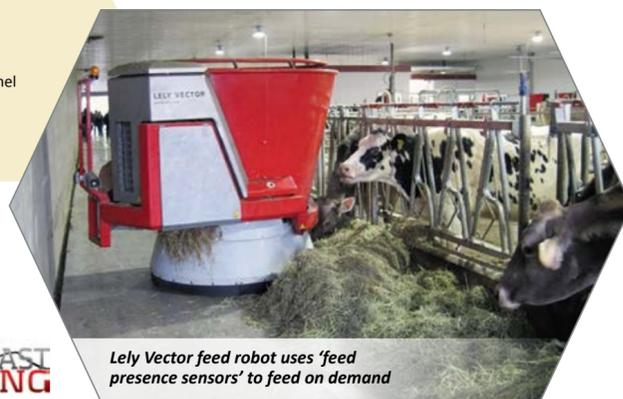
Lely Vector feed robot uses 'feed presence sensors' to feed on demand
